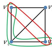
Figure 2. General Network: If the link  $(v_1, v_3)$  is removed from the original complete graph, we cannot get the measurement  $[1 \ 0 \ 1 \ 0] \mathbf{d}_{\mathcal{V}}$  any longer.
