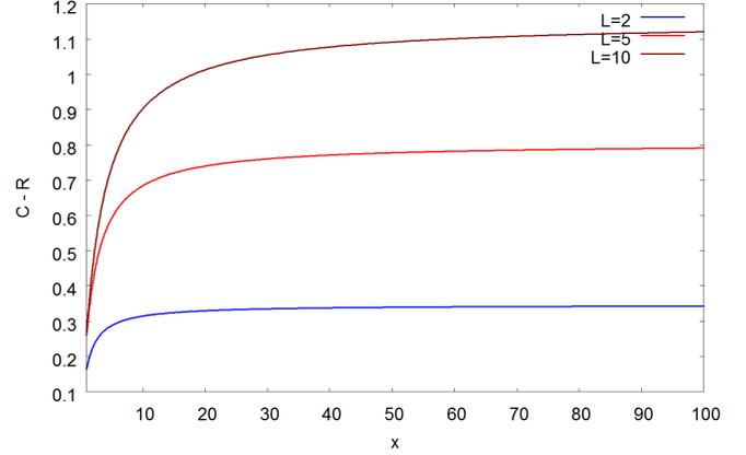
Fig. 3. For the ECGAL networks with equal channel gains: the gap between MAC cut-set bound  $C$  and analog network coding rate  $\bar{R}$  as the parameter  $x = \frac{Nh^2 P}{\sigma^2}$  increases. The number of nodes in each layer is  $N = 5$ . We observe that for a given number of layers in the network the gap approaches a constant value. As the number of layers in the network increases, the corresponding gap also increases.
