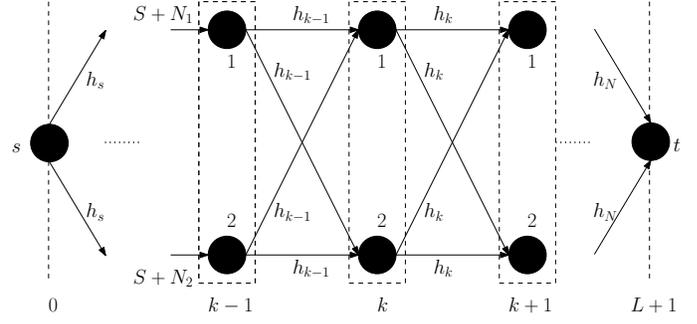
Fig. 2. An ECGAL network of  $L+2$  layers, with the source  $s$  in layer 0, the destination  $t$  in layer  $L+1$ , and  $L$  layers consisting of two relay nodes each between them. The channel gains along all links between two adjacent layers are equal.
