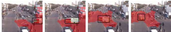
Figure 2: A fire engine (highlighted with a box) causing interruptions to left-right turn traffic flow. This anomaly is detected by the GP models because activity patterns from regions highlighted in red colour are contrary to the predictive distribution computed using the past observations from other regions.
